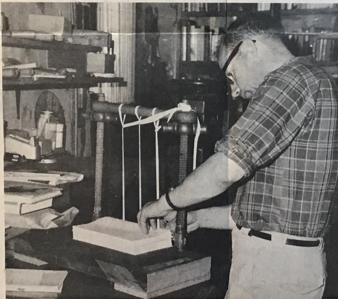
BOOK BINDER — Father Charles Brandt at his work-bench in his hermitage near Wolf Creek. He is shown in the initial stage of sewing Vatican Council documents prior to binding them. In the foreground is an altar missal he bound.
