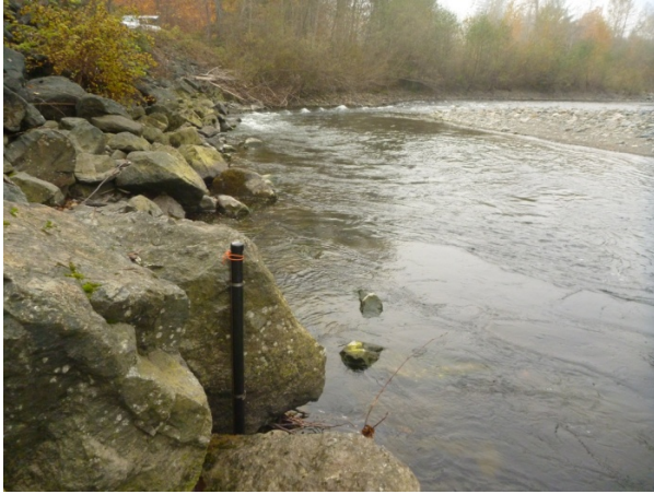
Photo 6. Upstream view of mainstem Oyster River water level logger (DLL-DS) installed in ABS pipe approximately 60 m downstream of the Connolly Sidechannel outlet. (Oct. 17, 2013)
