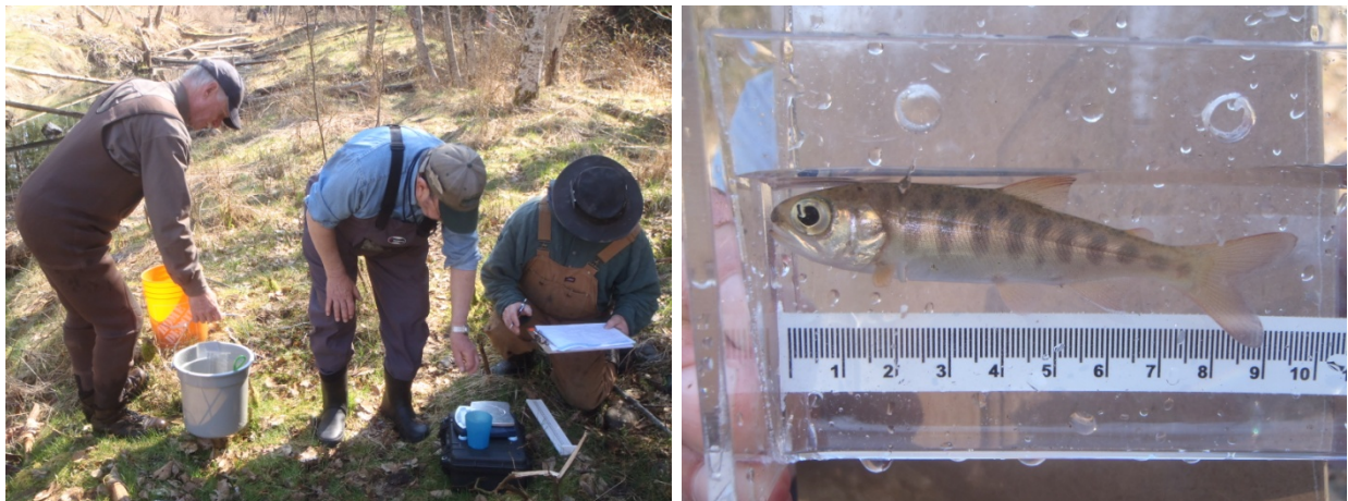
Photo 3 & Photo 4. Oyster River Enhancement Society Volunteers operating a digital scale used to acquire salmonids weights (above left) and a smolt board used to determine lengths (above right). (April 1, 2014)
