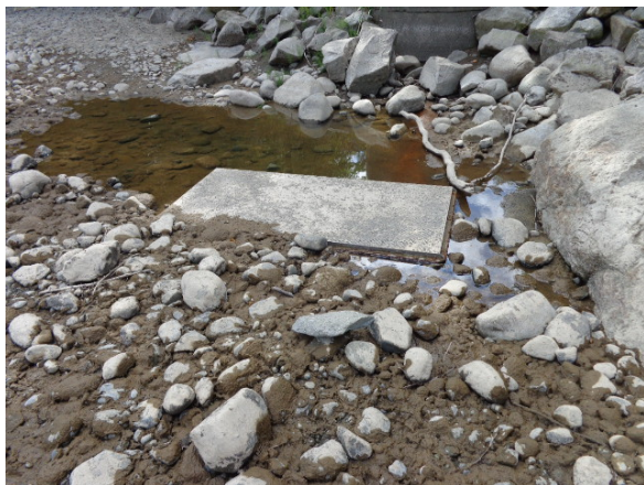
Photo 30. Mainstem intake screen showing dried condition beginning in August and persisting to the end of the study period in mid-September. (Aug.6, 2014)
